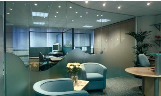
Sound reduction of up to 47 dB (Rw) can be achieved, whilst retaining the spacious, visual simplicity of glass. **Tenon Vitrage** is a double or single glazed partition system that combines function with the clear, aesthetic benefits of silicone glazing. Using a minimum number of aluminium framing sections, Vitrage provides an office divide that allows unhindered vision whilst maintaining the privacy of individual offices.
