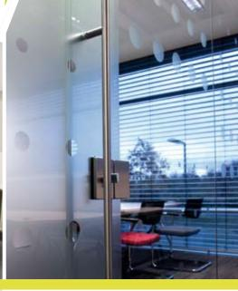
Gaskets and clear dry joints are used to hold the glazing in position which eliminates unsightly silicone and allows the partitioning to be demountable if required. Acoustic glass can be used to reach the maximum 47 dB (Rw) rating where it is essential to have optimum amount confidentiality or maintain a quiet environment.
